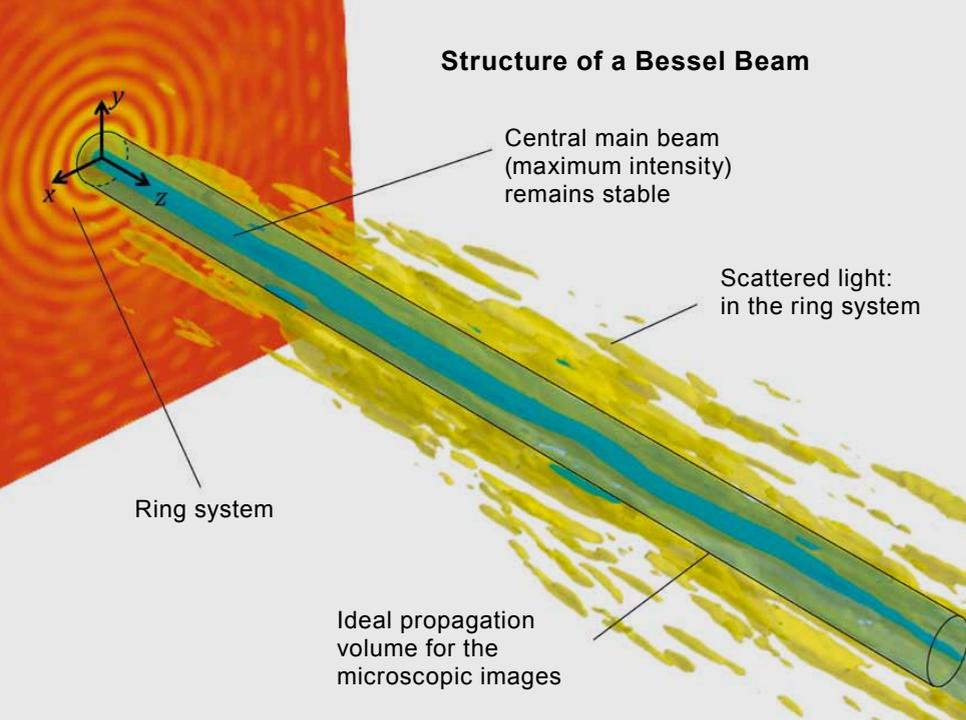
*Better contrast, higher resolution: The central main beam of the laser illuminates the object line by line. At the same time, a camera also captures the object as through a single-slit diffraction. This masks the light from the ring system.*
