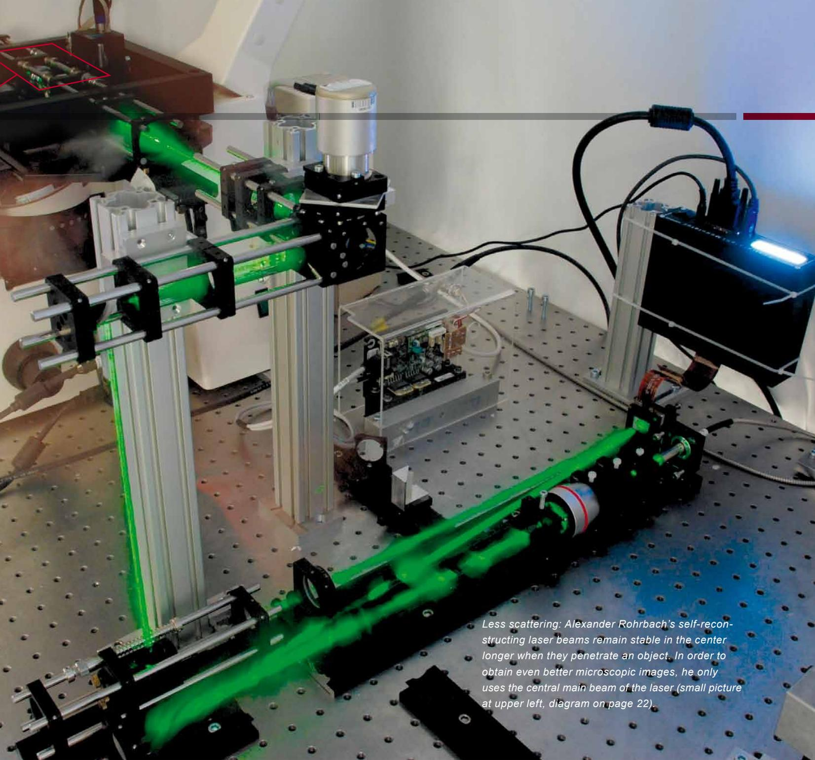
*Less scattering: Alexander Rohrbach's self-reconstructing laser beams remain stable in the center longer when they penetrate an object. In order to obtain even better microscopic images, he only uses the central main beam of the laser (small picture at upper left, diagram on page 22).*
