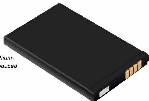
*Technically mature: Small-scale lithium-ion batteries are already mass produced for devices like mobile phones.*
