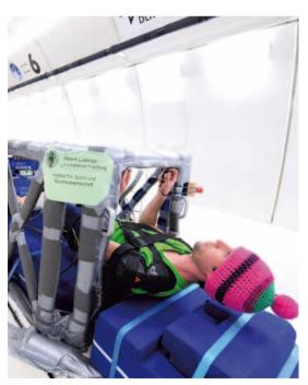
Whole body vibration, jumping, and balance control: The exercisers lie on their backs, their feet on a rectangular board. The machines simulate gravity by placing pressure on the shoulders. Photo: Hoffmann/Multhaupt DLR
