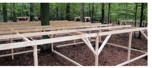
Covered up: The researchers are simulating drought in the forest with half-open roofs under the treetops. The picture shows how the roofs are built.
