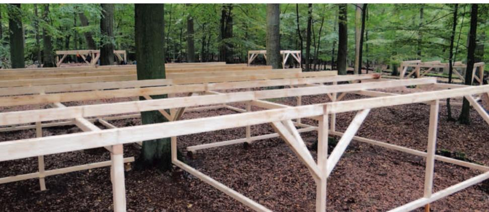
*Covered up: The researchers are simulating drought in the forest with half-open roofs under the tree-tops. The picture shows how the roofs are built.*
